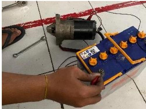
Gambar 14. Pengujian pull in coil.
