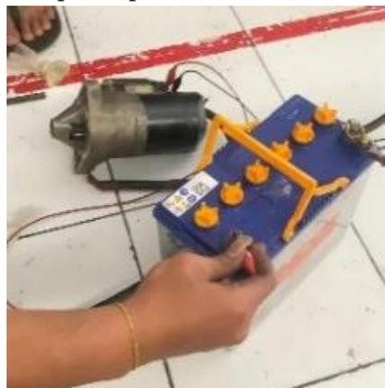
Gambar 15. Pengujian hold in coil.
