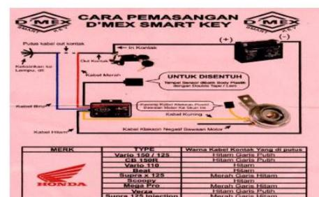
**Gambar 2.** Wearing Diagram Sistem Alarm
