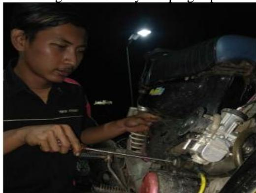
**Gambar 15.** Memasang Body Bagian Samping
