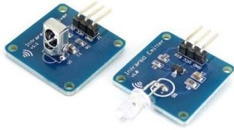
Gambar Transmitter Dan Receiver/ Detector Infra Red (<http://belajarelektronik.net>)
