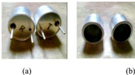
Gambar 2. Sensor ultrasonic (a) gambar sensor tampak belakang (b) gambar sensor tampak depan
