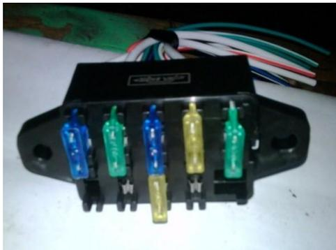
**Gambar 12.** Fuse box sekering
